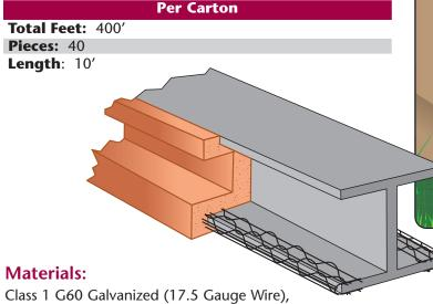
Class 1 G60 Galvanized (17.5 Gauge Wire), Stainless Steel (17.5 Gauge Wire) 316L Stainless 18% Chromium
