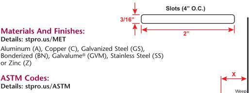
All Accessories are fabricated from prime galvanized steel G90 zinc coating by the hot dipped method, conforming to steel and coating specification ASTM A-653/A-653M or zinc alloy meeting ASTM B-69. Stainless Steel A480/A480M A580M (Stainless Steel) For installation and placement
