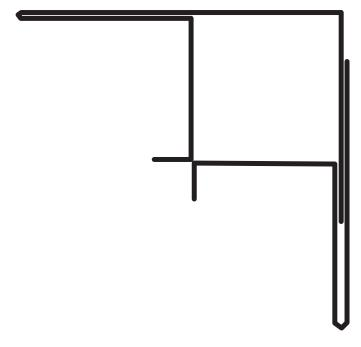
Designed to facilitate movement at an inside corner condition.
