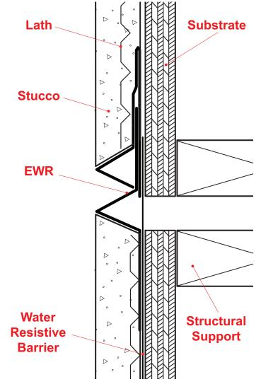
The dual function self-aligning expansion joint provides movement capability at floor line while allow moisture to release from the top ground and locks out moisture from the bottom. Special "Step" on the attachment leg provides a locator for correct placement of the fasteners and helps keep the molding laying flat on the wall.
