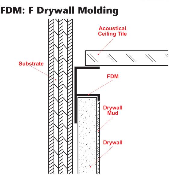
A drywall stop/control screed for drywall, used at the top or base of columns, the top of walls at the ceiling, or at the base to create a reveal. Also used at the top of windows to permit the continuation of a horizontal reveal at the window line.
