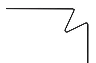
Use this product when needing a straight, clean inside edge at a vertical or horizontal corner. Provides a straight edge where soffit and wall meet.
