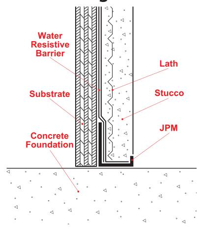
A plaster stop/casing bead for conventional 3-coat stucco used in a variety of conditions that gives a nice finished look at all plaster terminations.
