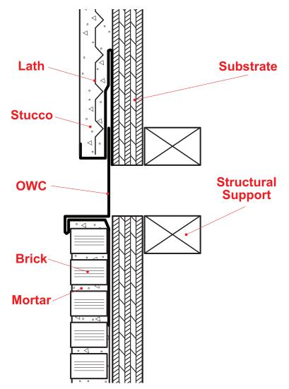
The OWC is the same as the EWC except that it offers two leg lengths for situations where 2 dissimilar depths come together. Special "Step" on the attachment leg provides a locator for correct placement of the fasteners and helps keep the molding laying flat on the wall.
