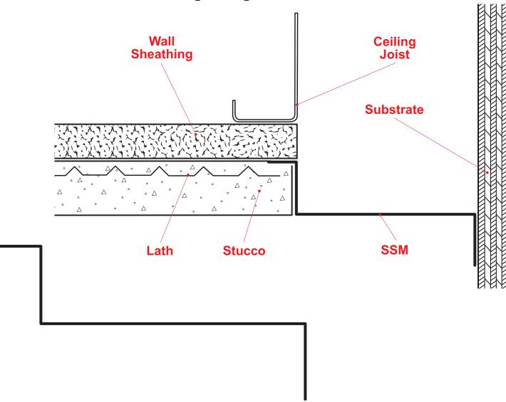
A versatile molding used primarily to separate either plaster or drywall from other materials.
