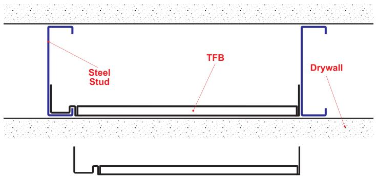
Low profile, return lip backing that provides increased load capacity. TruFlush™ Backing will eliminate build up, drywall cracking and drywall fastener popping. Available in 20 gauge or 16 gauge for 12", 16" and 24" stud spacing.
