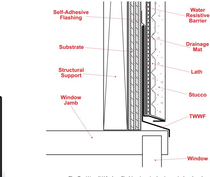
The Tru-Weep™ Window Flashing is a single piece window head flashing weep specifically designed to be used with drainage mat. Weep slots are located along the back of the sloped leg in alignment with the drainage mat to allow water to efficiently exit the stucco assembly.
