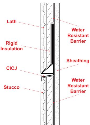
CICJ is a drainage point control joint for CI (continuous insulation) stucco assemblies. The ground points can be customized to accommodate any combination of rigid insulation and stucco CI system. Available with or without weep holes.
