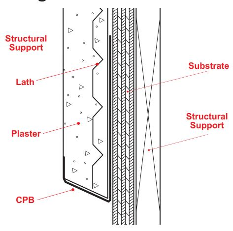
A plaster stop/casing bead used to terminate the stucco at the base of walls and/or where a plaster stop is required. Has a 60° angle which creates a unique look.
