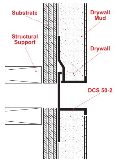
A two-piece version of the DCS series molding that provides 3/4'' +/- movement where a "true" expansion joint is required. Used for stucco over block or when only a 1/2'' depth is required.
