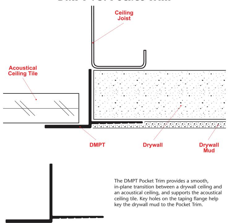
Note: This drawing is supplied solely to assist in the selection and application of product manufactured by Stockton Products. This drawing is generic in nature and should not be used in design or construction without an independent evaluation by a qualified Architect or Engineer of Record.
