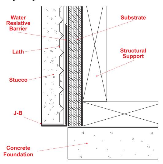
Standard plaster stop/casing bead for terminating stucco. Has a return key for finishing.
