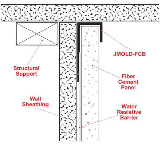
Used as a termination molding to case off the fiber cement panel.
