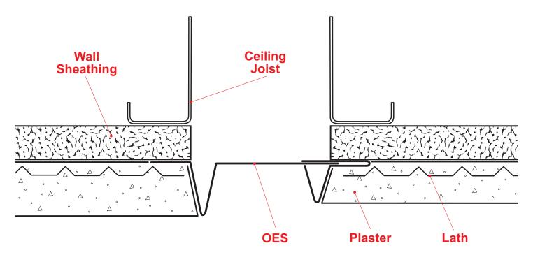
Adjustable version of our Offset Reveal Screed that permits movement in a double stud condition and at floor lines. Available vented for air flow.
