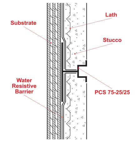
Plaster channel screed with minimal reveal width and ground depth for conditions that require a control joint with a small reveal.
