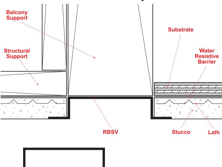
A removable soffit vent that permits access to the balcony soffit space for inspection at the balcony/wall transition and allows for free air movement and ventilation. Complies with the City of Berkley R1 and R2 Zoning Districts for Exterior Elevated Elements. The soffit vent is easily installed and removed. 1/2" wide return legs are provided that will cover the rough opening.
