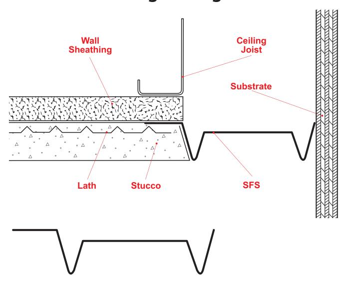
Same as our standard vent, less one flange, designed to butt against walls on one side while providing a plaster stop on the other. Can be used in ceiling/wall or base conditions providing perimeter airflow. Available non-vented for use as a decorative reveal upon request.
