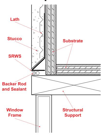
The #6 Solid Return Weep Screed in an angles drip screed that can be used at base of walls. It may also be used as a window or door head plaster stop and flashing piece.
