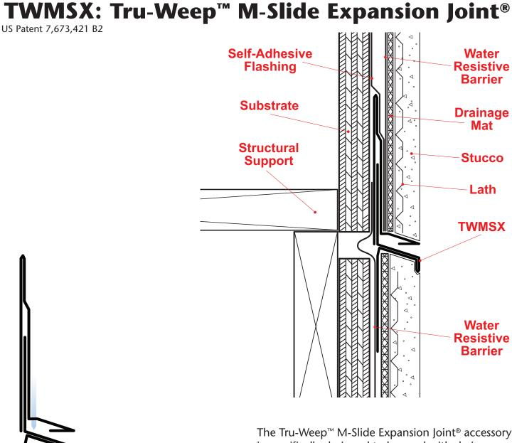
The Tru-Weep™ M-Slide Expansion Joint® accessory is specifically designed to be used with drainage mat. Weep slots are located along the back of the sloped leg in alignment with the drainage mat to allow water to efficiently exit the stucco assembly.
