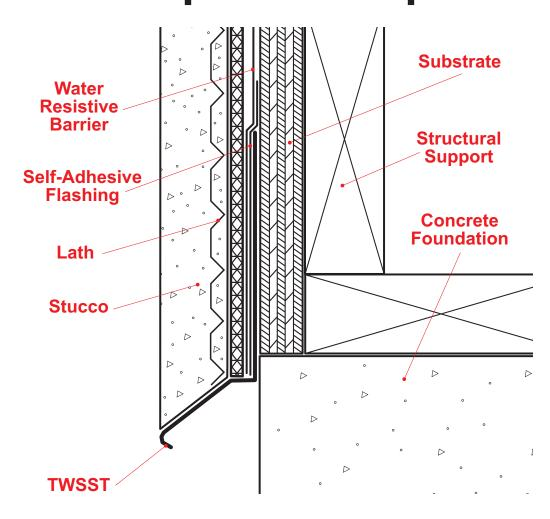
The Tru-Weep™ Stucco Stop is a single piece variation of the traditional weep screed that provides a plaster stop and weep function at the foundation line, and specifically designed to be used with drainage mat. Weep slots are located along the back of the sloped leg in alignment with the drainage mat to allow water to efficiently exit the stucco assembly.
