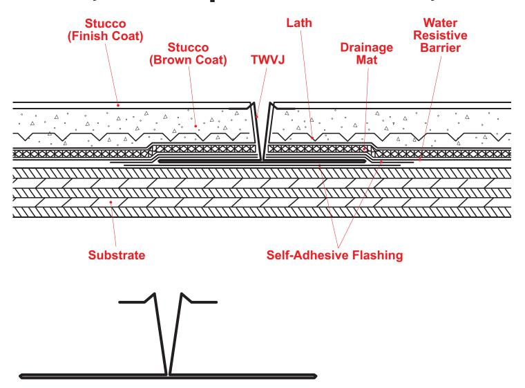
The Tru-Weep™ Vertical Control Joint is a customizable vertical control joint specifically designed to be used with drainage mat stucco assemblies. Tru-Weep™ Vertical Control Joint is to be used with drainage mat stucco assemblies per 2021 IBC: 2510.6.1
