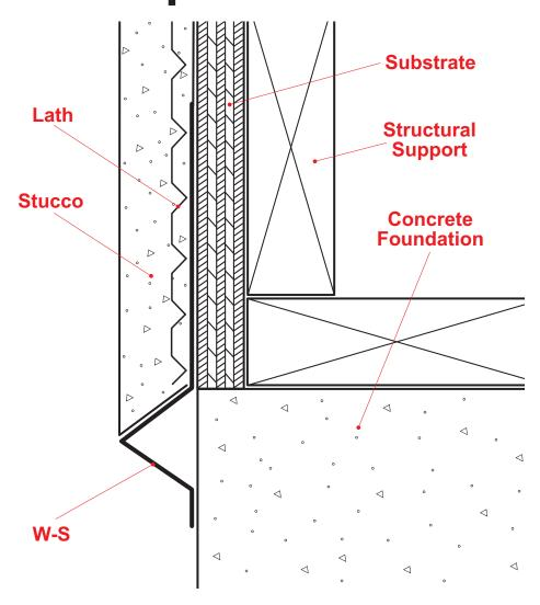
A traditional weep screed that provides a plaster stop and functions as a weep screed at the foundation. Available with and without weep holes.
