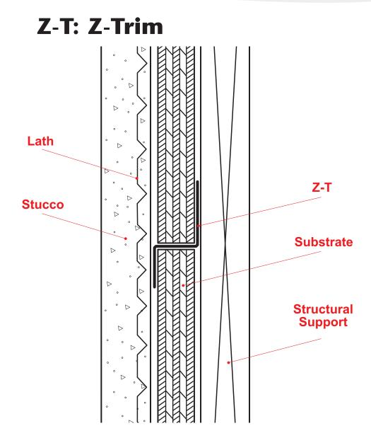
Used to properly seal and join two pieces of plywood and other conditions where a "Z" shape is required.
