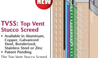
The Top Vent Stucco Screed is a single piece vented plaster stop specifically designed to be used with drainage mat to efficiently allow water vapor to escape through the concealed air slots.
