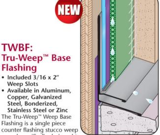
screed specifically designed to be used with drainage mat transition points between dissimilar claddings. Weep slots are located along the back of the sloped leg in alignment with the drainage mat to allow water to efficiently exit the stucco assembly.
